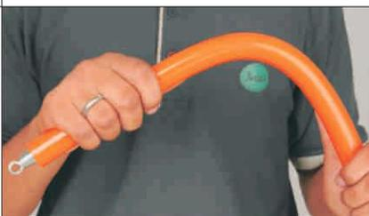
The pipe is bended using internal bending spring. The Aluminum makes the pipe form-stable (i.e. non spring-back after bending) & impermeable to oxygen diffusion. Once bent, the pipe maintains its shape.
