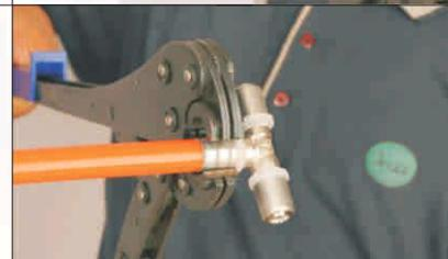
**Joining Procedure for Press Fittings (crimp-fit)**
